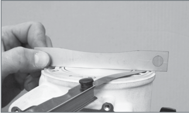
Case where the piston pushes the plate causing cylinder/plate contact to be lost
