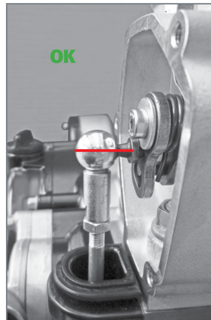
Correct position of the control rod seat.
