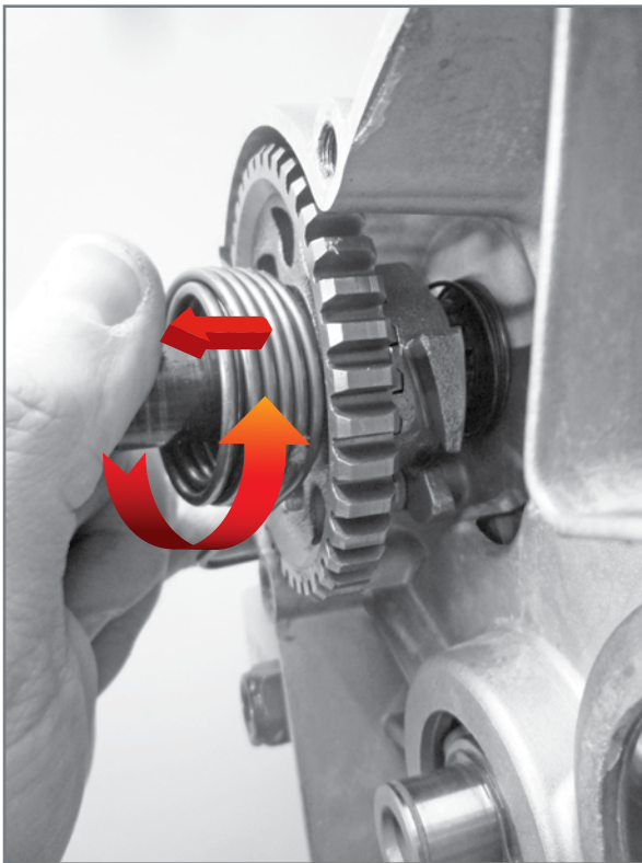
Extraction of shaft from crankcase.
