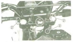
Tighten the ring nut using the ring nut wrench.
